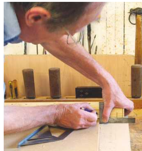
Pic.13 Mark the edge of the fence with a square
